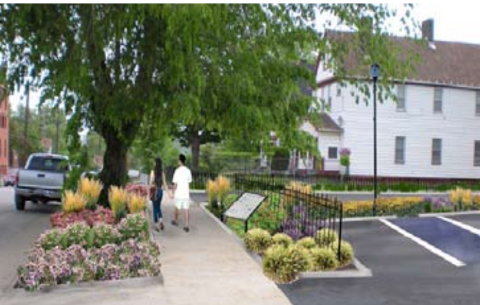
Illustration of a parking lot in Tremont neighborhood designed to provide bio-retention areas for managing stormwater; Illustration by: Katherine Holmok
